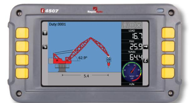
One of the latest tower crane software developments is the swan neck tower crane software. The software uses both unladen and laden radius calibrations to ensure the readings are always accurate. This coupled with load, angle and wind speed monitoring gives the i4500 a full view of the cranes safe working parameters. For more information please contact RaycoWylie.
