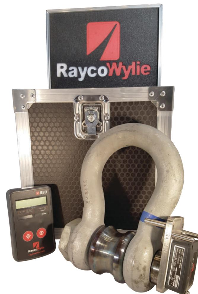
Raycowylie offer the W890 range of load shackles, ranging in capacity from 6.5te to 35.0te. The load pins are manufactured from 17-4 stainless steel for strength and reliability, these shackles should be used with the appropriate bobbin to ensure the load is directly applied to the centre of the load pin therefore giving the most accurate results.
