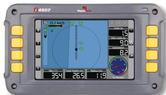
The prohibited zone function allows to limit access of the jib or trolley and lifted load to different zones without losing sight of the critical load information. You get one zone to determine the job site and up to ten zones (3D) to determine obstacles inside the jobsite.
